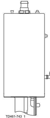
Actuator for the change-over valves can be reversed from NC to NO and from NO to NC.
