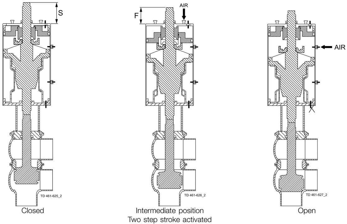
The plug opening for different change-over valves and actuator size is shown below.
