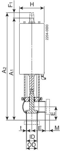
Figure 1. Shut-off valve
