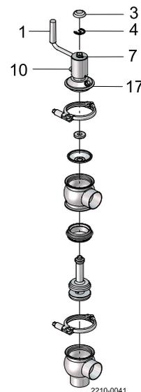
Make sure that the diaphragm is securely mounted on the sealing element (17), before installing the complete diaphragm, disc and spindle into the valve body.
