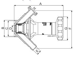
Figure 1. Handle with valve body: Collared pipe welding
