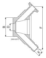
Figure 4. Valve body: Tank welding
