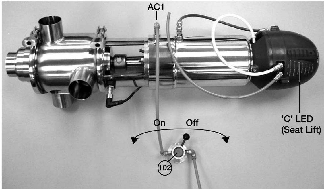
1. Valve at rest (closed) position
