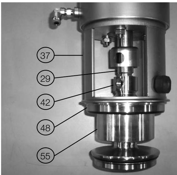
13. Fit upper plug (55), upper sealing element (48) and spindle liner (42) into intermediate piece (37).
