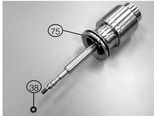
20. Remove O-ring (38) from lower plug stem (75).
