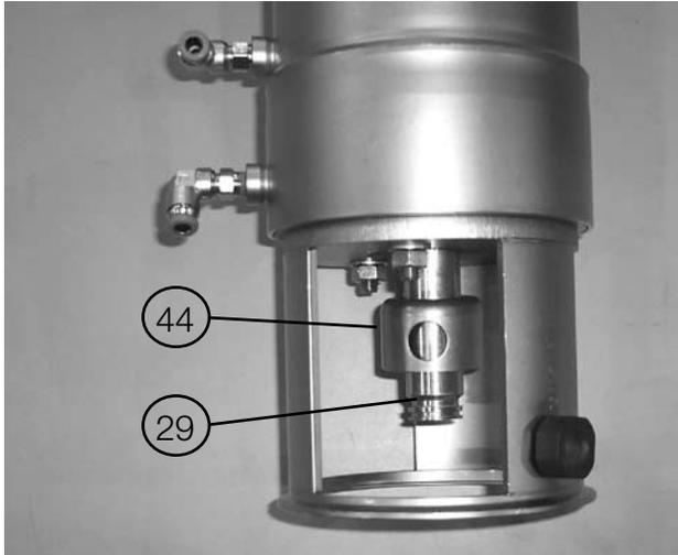
10. Install lock (44) onto piston rod (29).
