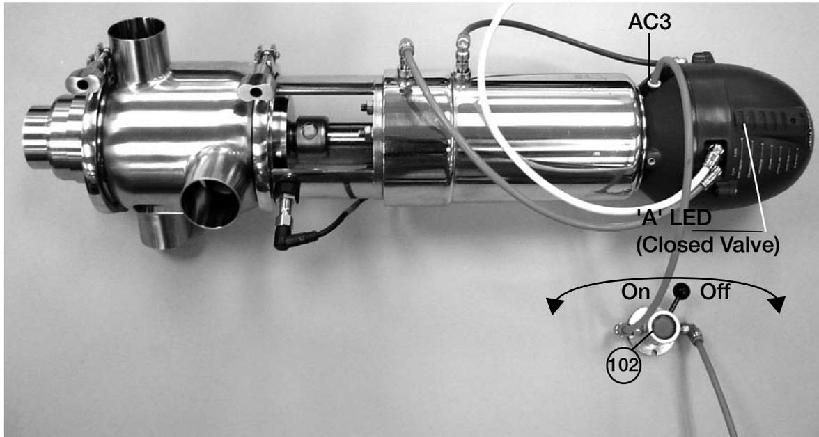
1. Valve at rest (closed) position
