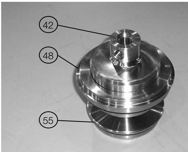
11. Slide upper sealing element (48) onto upper plug (55).
