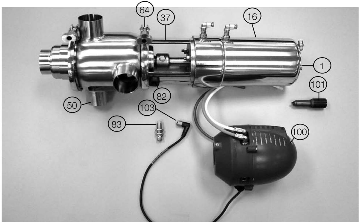
34. Turn sensor (83) clockwise into nylon plug (82) and tighten by hand.
